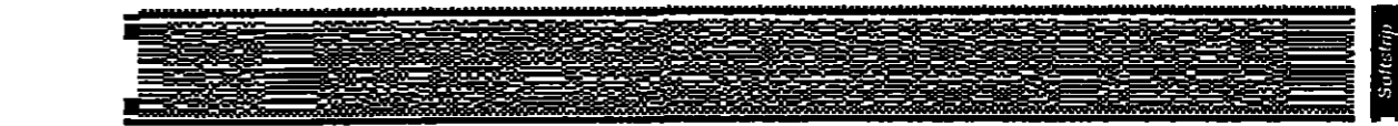
THIS STRIP CONTAINS AN IBM BASIC PROGRAM THAT LETS YOU USE YOUR PC AS A SKETCH PAD.
